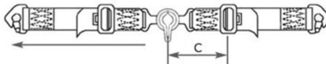
Length C:  Standard Length of Dimension 'C' Pull Up or Pull Down is 6" (150mm) Centres
